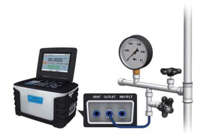
Figure 3-20 Calibrating a dial pressure gauge
