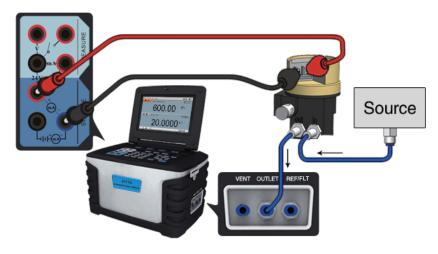
Figure 3-24 Calibrating an I/P converter
