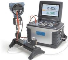
Figure 3-3 Gauge pressure source
