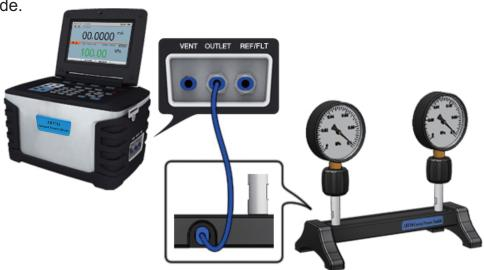
Figure 3-16 Calibrating pressure gauges
