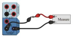
Figure 3-7 External power supply
