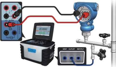
Figure 3-17 Calibrating a pressure transmitter
