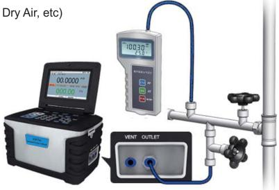
Figure 5-1 Calibrating a digital barometer
