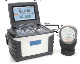
Figure 3-4 Differential pressure source
