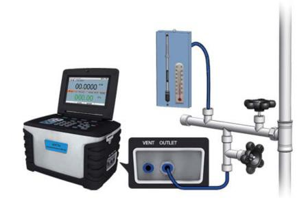
Figure 5-2 Calibrating a mercurial barometer
