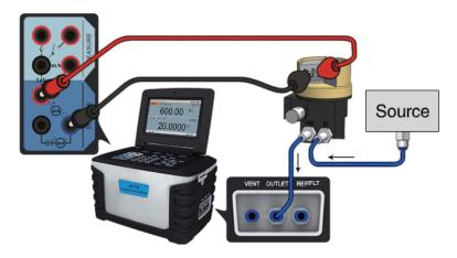
Figure 3-19 Calibrating a I/P converter
