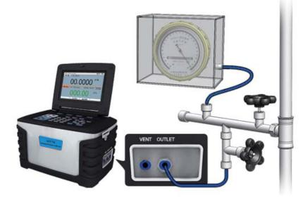
Figure 5-3 Calibrating an aneroid barometer
