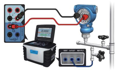
Figure 3-22 Calibrating a two-wire pressure transmitter
