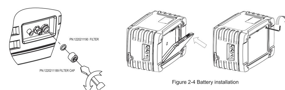
Figure 2-3 How to change filter
