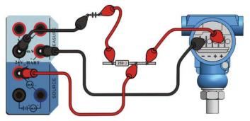
Figure 3-15 External series resistor and external loop power supply
