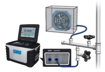
Figure 5-4 Calibrating a barometer altimeter
